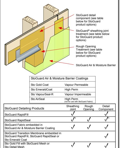
\* StoGuard RapidSeal requires StoGuard Mesh or Sto Detail Mesh embedded when used as sheathing joint or
